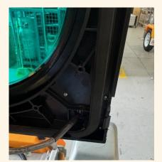
**Step 11:**Replace the rubber seal
